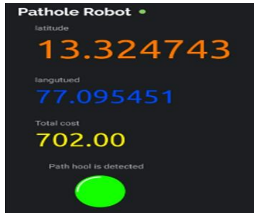
Fig 4 Real-time pothole detection and data transmission via the Blynk IoT platform
