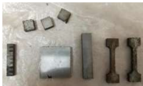
Fig. Inconel625+SS304L Specimens after Wire EDM cutting
