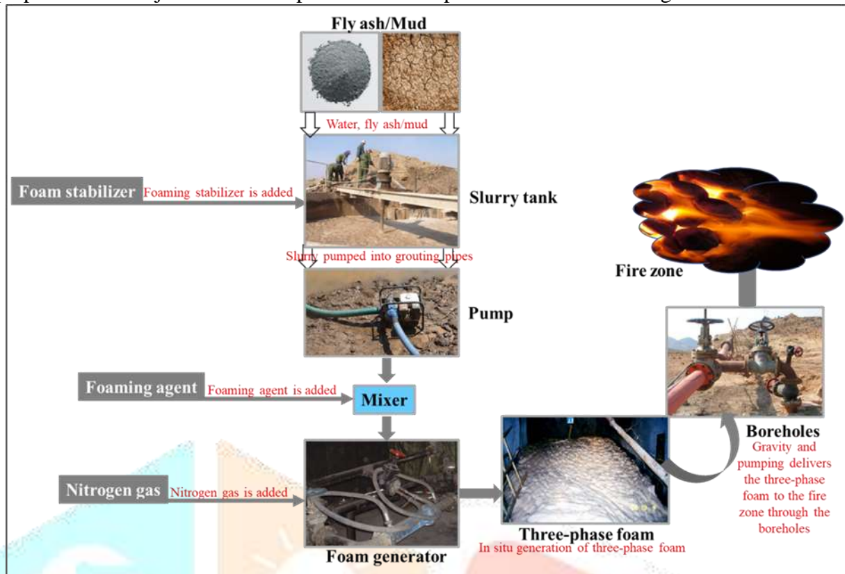
Fig. 4-2 Three-phase foam preparation and injection into the underground fire zone, modified from [13]
