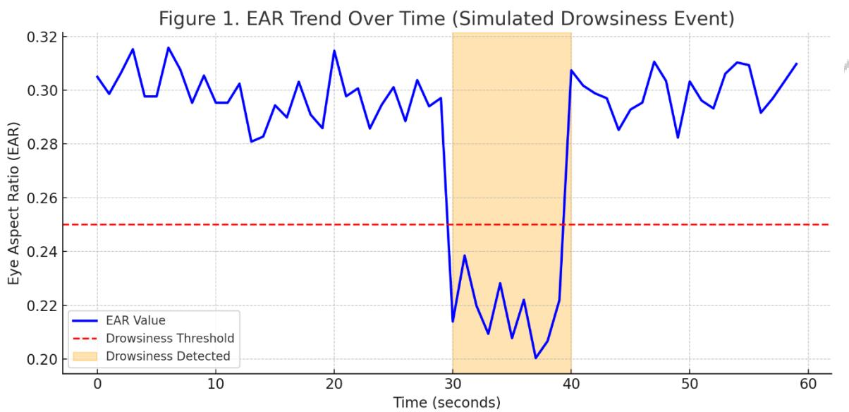
This temporal reduction, which is defined by successive low EAR values, triggers the alarm mechanism. Adaptive thresholding prevented false alarms due to natural blinks or transient closures.
