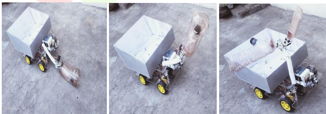
Figure 6: Robotic Arm in action during waste collection
