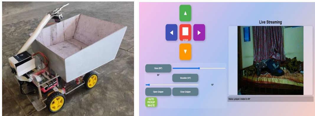
Figure 5: The complete assembled waste collection robot and controlling web page Live View
