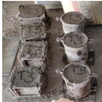
Figure 2: Casting of cubes, cylinders.
