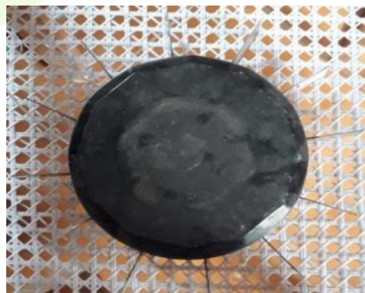
Figure 5: (Image of aluminium finned cooking pot with black painted pot)
