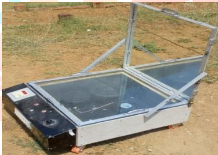
Figure 8: (Box type solar cooker with fan in cooking space)
