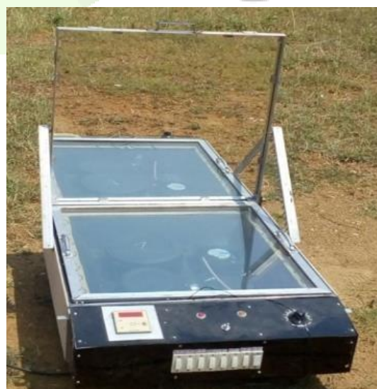
Figure 9: (Experimental set up of a box-type solar cooker)
