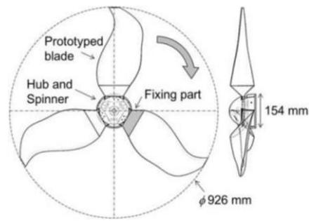
**Fig.4. Biomimetic Wind Turbine**
