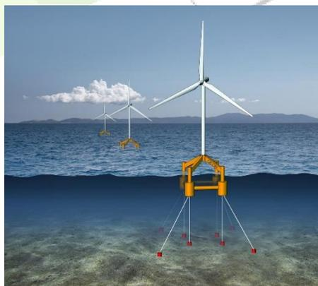
**Fig.3. Floating Wind Turbine**
