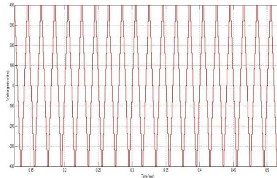
Fig 15 Simulation Output Voltage Waveform of A new eleven levels with reduced switches MLI with PWM Technique
