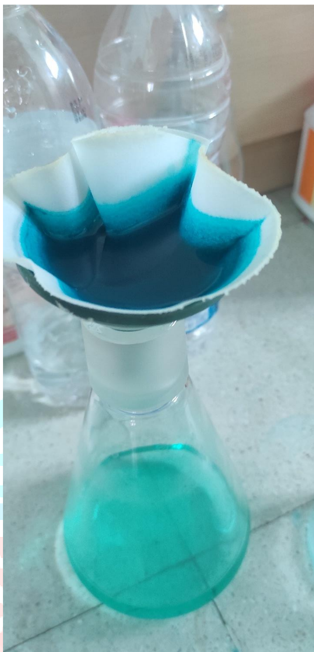
Using Whatman Filter Paper No.42 To Filter To Filter The Acidified Precipitate.
