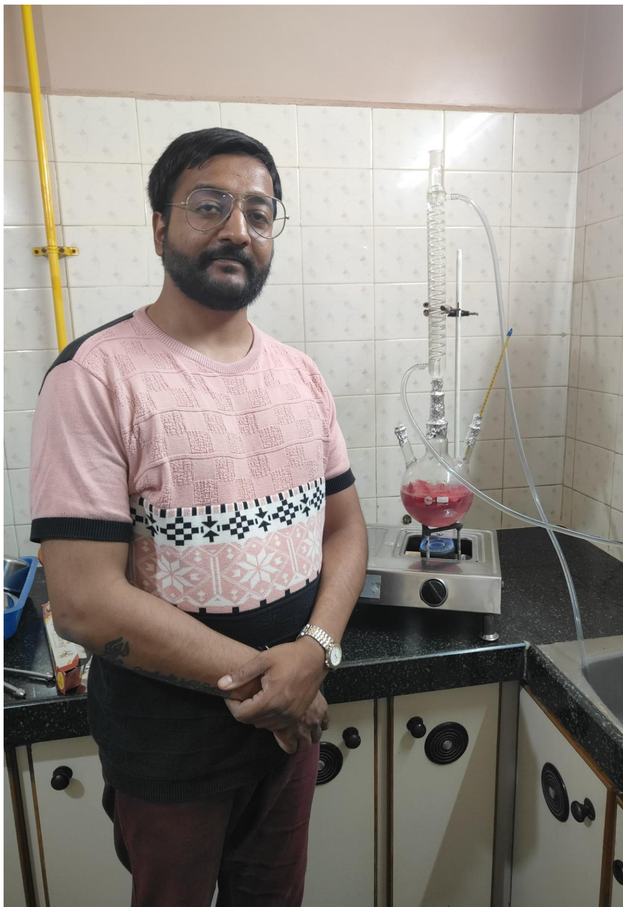
Set Up for Laboratory Extraction Through Reflux Condenser.
