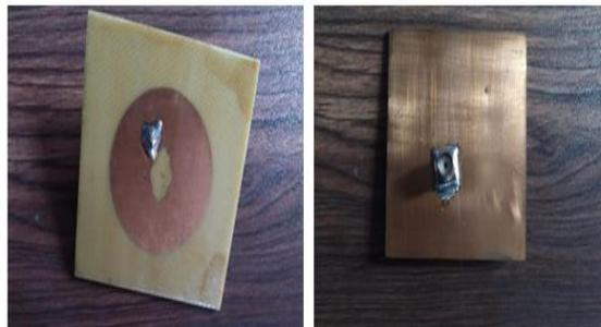
Fig.10 fabricated antenna prototype
