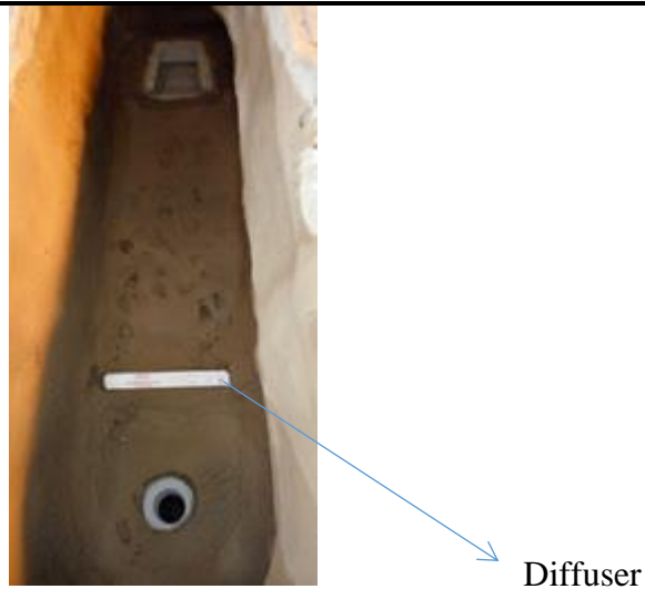
Fig. 3 Diffuser applied at the bottom of tundish
