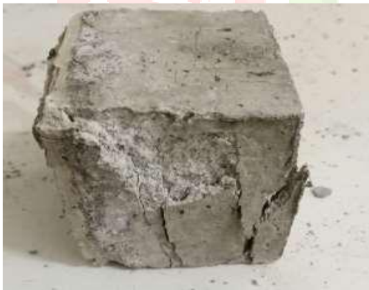
Fig. 2.11 Cubes failed under compression
