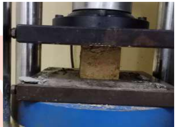
Fig. 2.10 Cube placed in CTM
