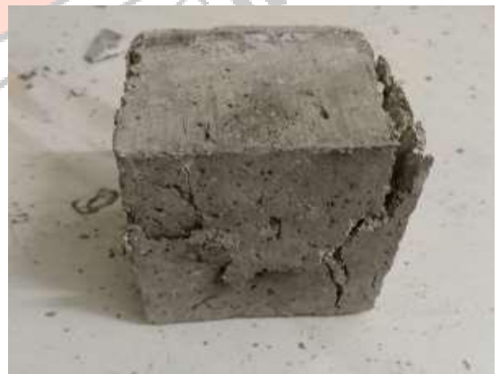
Fig. 2.10 Cube placed in CTM
