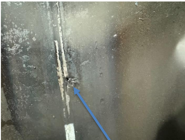
Figure (3)-volumetric defect (visual hole) on weld (ID)
