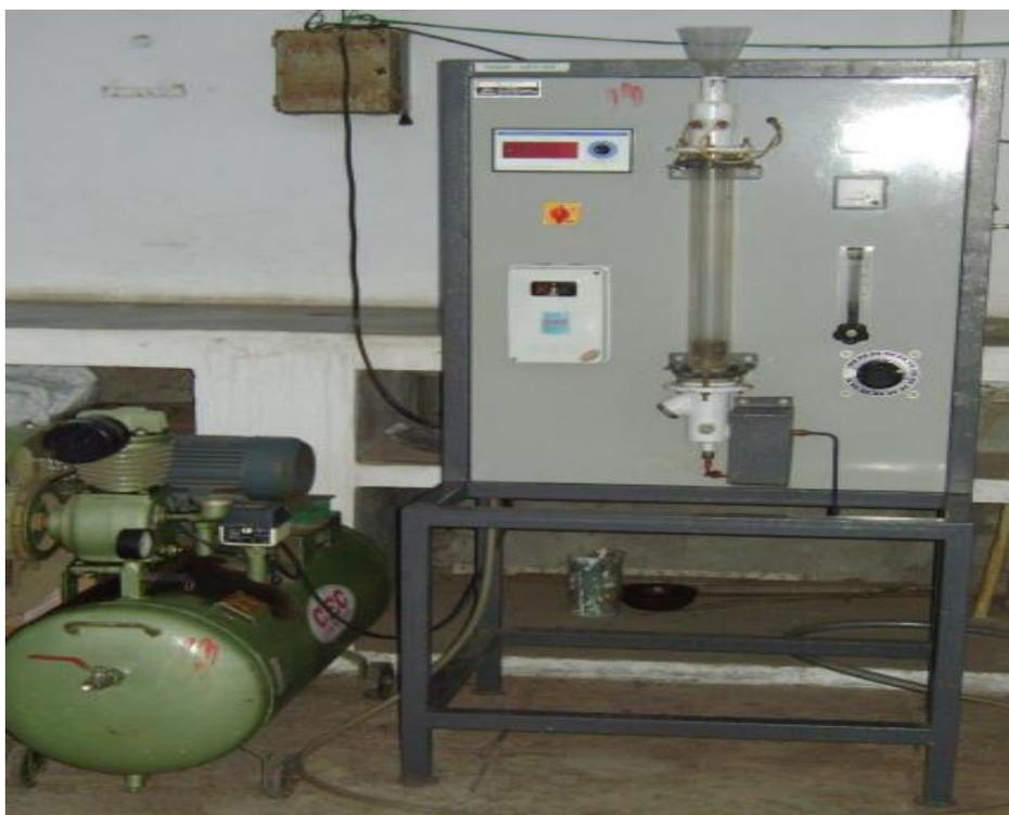
Figure:1 Fluidized bed dryer set-up
