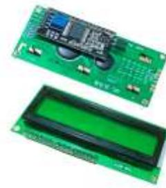
Fig 3: LCD display16X2
