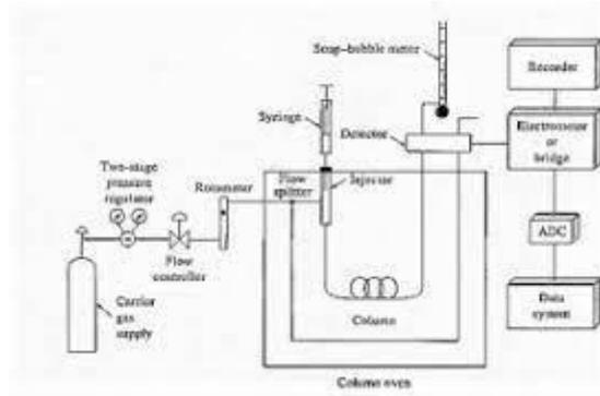
“Fig: -1” Schematic diagram of gas chromatography
