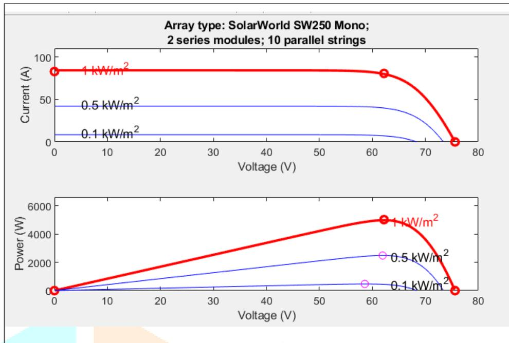
Figure 7: PV array output voltage vs current and voltage vs power graph.
