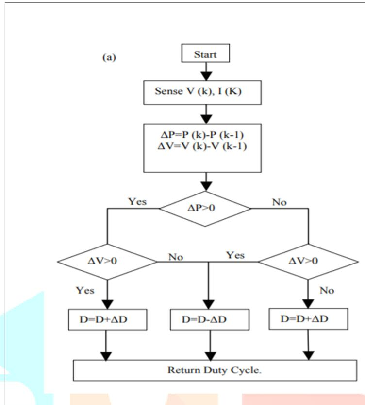
Figure 1: flow chart of MPPT algorithm.
