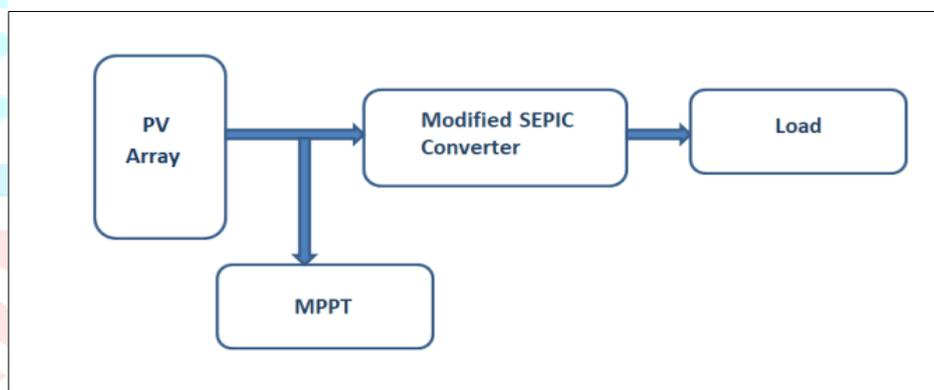
Figure 5: Block diagram of proposed system.
