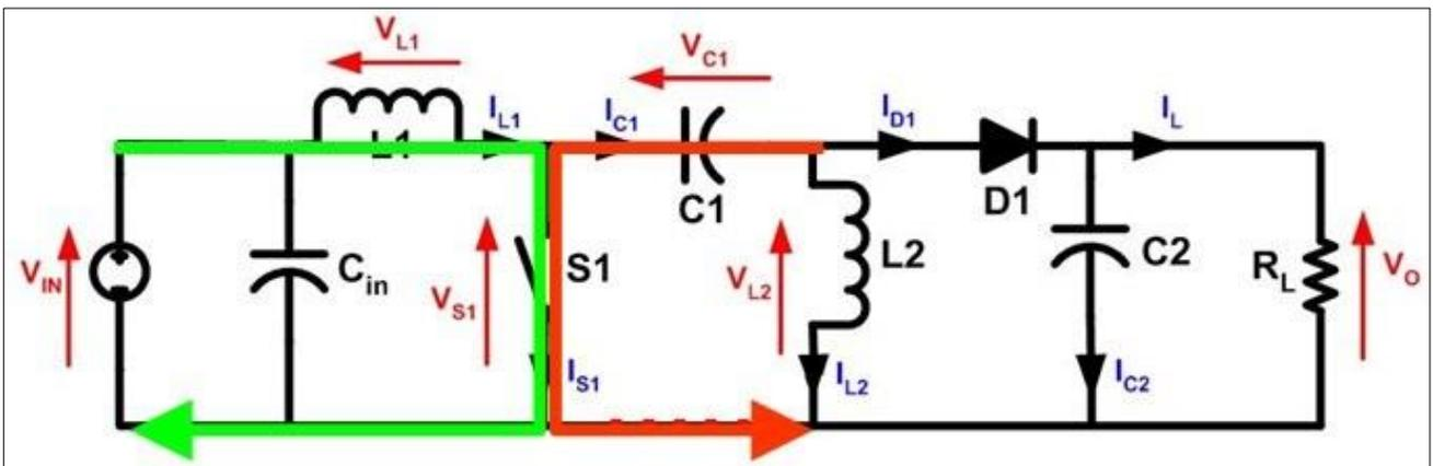
Figure 3: when IGBT is ON then current flows through L1 and C1 also discharges current flow from L2.
