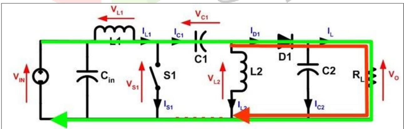
Figure 4: With S1 open current through L1 and current through L2 produce current through the Load
