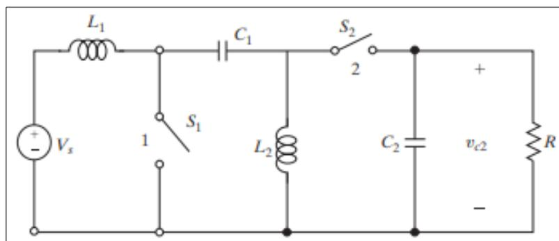
Figure 2: Basic block diagram of SEPIC Converter.
