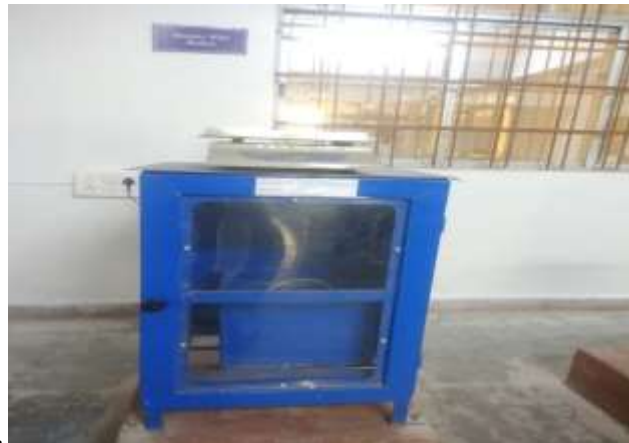
Figure: 2.6 : Specific Gravity & Water absorption test machine of coarse aggregate
