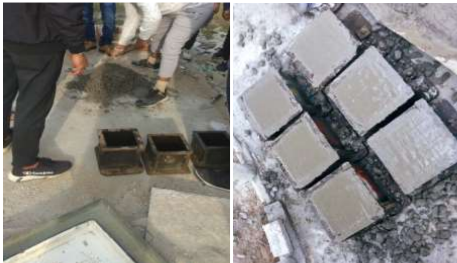
Figure: 2.7 : Casting of cubes
