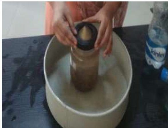
Figure: 2.4: Specific gravity test of sand
