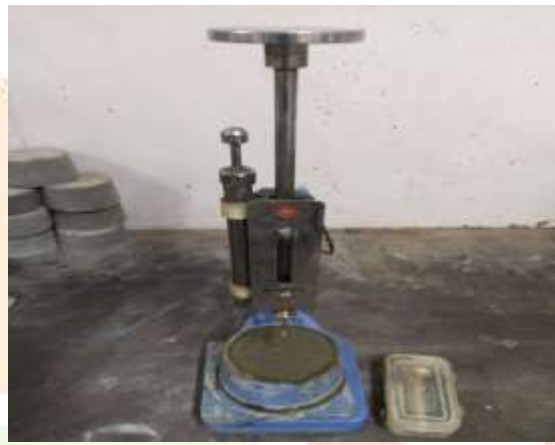
Figure: 2.3 : Vicat Apparatus for Consistency, Initial setting time & Final setting time test of cement
